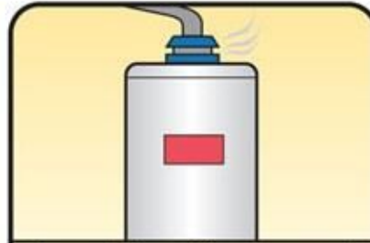
Corroded or Disconnected Water Heater Vent Pipe
